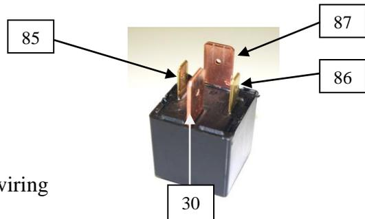
Now, with relay unplugged, check across terminals 85 and 86 of the relay, using an OHM meter. You should have approx. 80 to 100 ohms. This is measuring the resistance through the relay coil. If you do not, replace relay.
