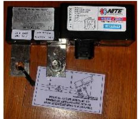
Example 1. If the fuse blows and the solenoid is engaged, the start batteries and the auxiliary batteries will stay connected until the fuse is replaced and the voltage allows it to reset. This allows the possibility for the truck batteries to be discharged and the truck may not start.
